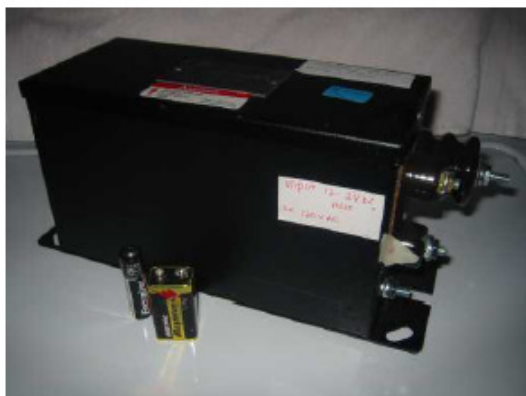
15,000 v Neon Transformer
