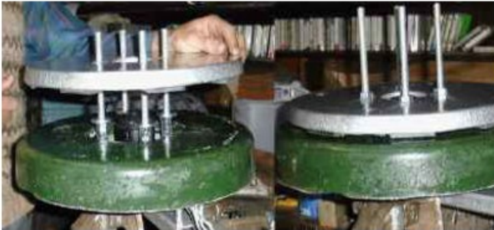
Fitting the front magnet rotor
