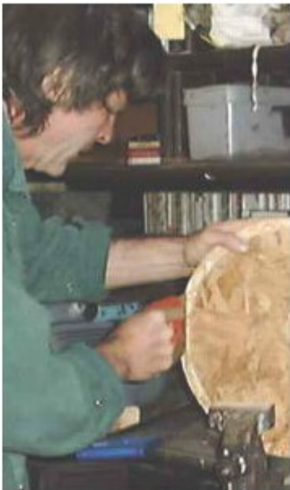
Sawing flat faces on the inner mould
