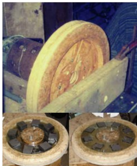
Rotor mould being made and used
