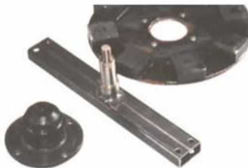
Spine, shaft, hub and magnet rotor
