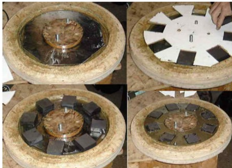
Four stages of the rotor casting procedure
