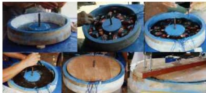
Six stages of the rotor casting procedure
