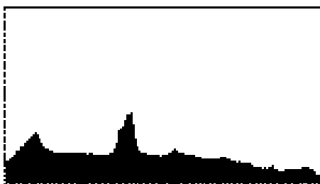
Metal-halide HID lamp POWERSTAR HODS® CRI 92 / 5,120-6,000K (daylight)
