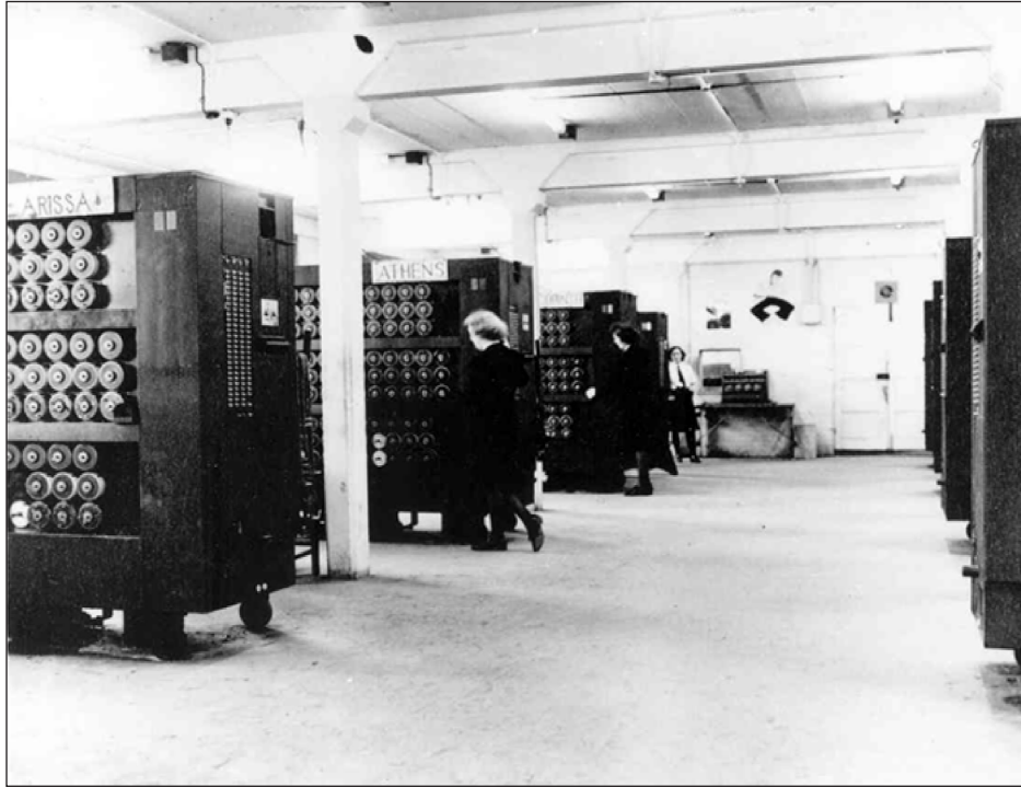
UK bombe deck. The United States would build its own version of the bombe for work against the four-rotor Enigma based in part on the British experience using these machines.
